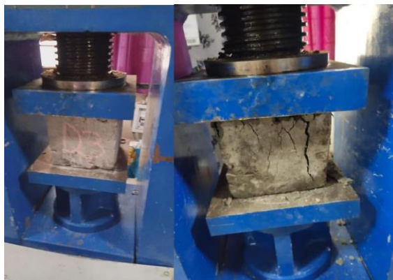
Fig 3.8: compressive strength test on concrete
